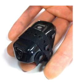
When properly fastened, the fabric strap will cover the eVu TPS device logo, but the indicator light will be visible when the device is on.
